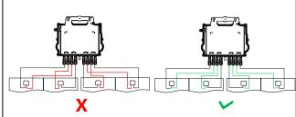
Step 8. Connect APsystems Microinverters to Grid
